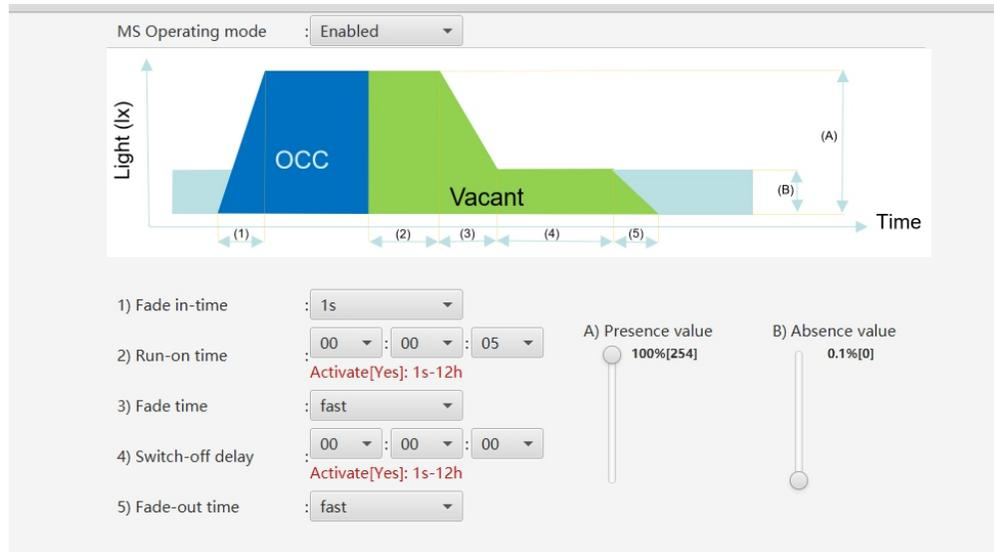
**(1) Fade in time:** this means the time that the destined DALI luminaires take to fade from current state to the configured state when the movement detected and the room is occupied.
