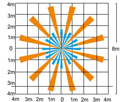
The detection area for movement sensor can be roughly divided into two parts:
